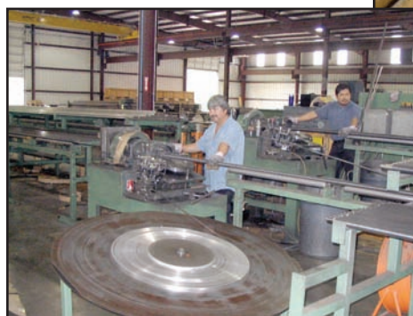
Employees at Vulcan Finned Tubes produce the aluminum L-foot finned tube.
